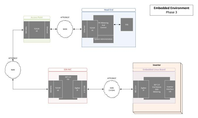
Figure 2. Embedded Environment - Inverter Deployment to the Embedded Environment [SSN SoW Task 1.3]
