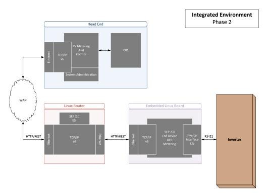
Figure 1. Integrated Environment - Inverter Deployment to the Integrated Environment [SSN SoW Task 1.2]
